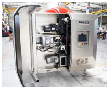
Nuova cofanatura vano motore. New bonnet of engine compartment.
